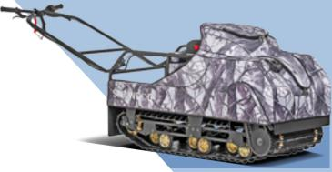
**SnowDog Standard** is a reliable companion designed to take you long distances in deep snow pulling loads of up to 650 lbs³. With its longer track and frame, Standard models offer you improved off-road performance and more cargo space. I comes equipped with powerful 10 hp or 13 hp Briggs&Stratton engine and a CVT. SnowDog Standard can overcome ice tracks, deep snow and harsh landscapes. Standard equipment includes LED light, electric starter, disk brakes and convenient engine cover.
